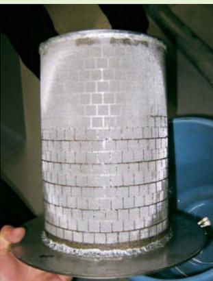
After 30 seconds\* of high-pressure jet cleaning, the filter has been cleaned.
