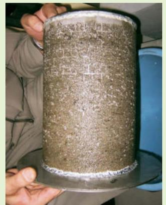
Foreign particles thickly-sedimented on the filter.
